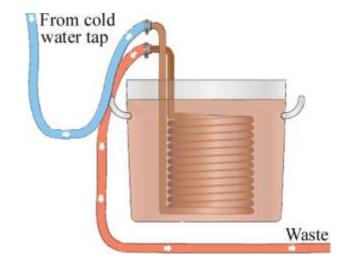
I have seen (too) many books, magazines & websites of wort coolers/chillers displaying the wrong set-up, i.e. the inlet & waste pipes connected the wrong way round.
